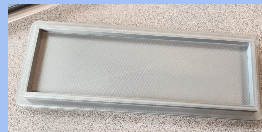
This is the cover for the case and is a friction fit as of now, but changes could be made in the future.
