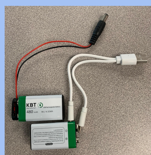
Our two batteries and a charger for them. Also the battery cable for the arduino is connected.
